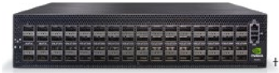
Figure 15. NVIDIA SN4600 switch
